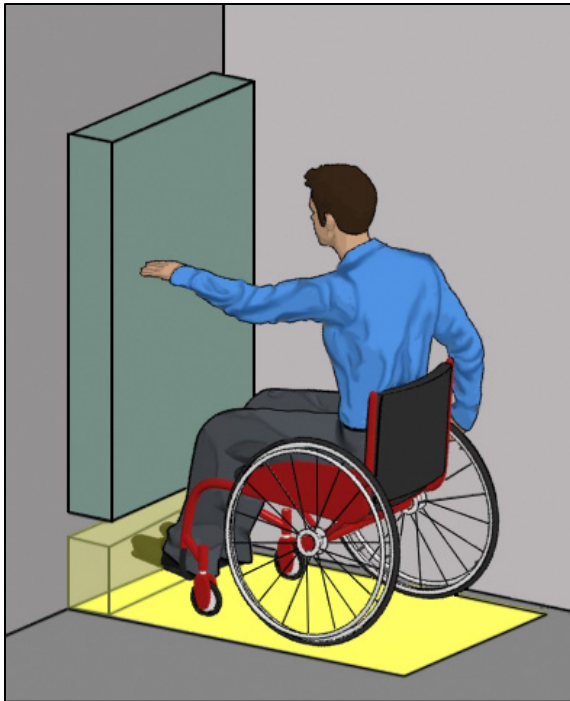
Toe space (9" high min.): Max. depth 6"
