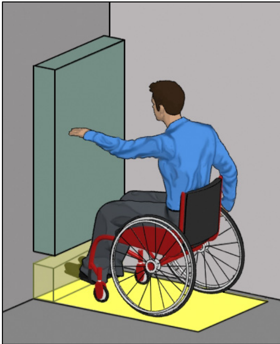
Toe space (9" high min.): Max. depth 6"
